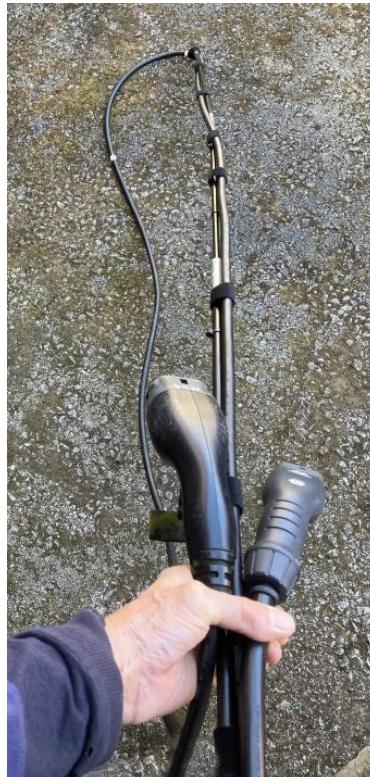
36. Check that the cable can reach the car without bending the top wand below horizontal, and adjust the arrangement as necessary. You can have more than 2.5 metres of cable extending beyond the wands if appropriate.
