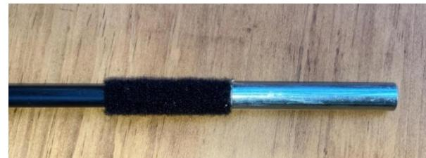
13. Wrap piece B of Velcro around a short wand 45mm from the plain end (the end without a metal ferrule).
