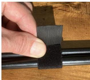
22. Use the 30mm wide wraps to attach the cable to the tip of the wands, and then over each of the 20mm Velcro tapes at 28cm intervals. Choose the side of the wrap that sticks to the previously fixed Velcro tape. (This stops the Velcro wraps slipping downhill when the assembly is lifted up.)
