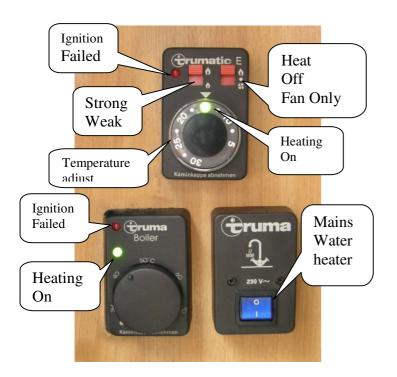
If the blown-air heater fails to light the red light glows. Give it a few minutes and try again. This heater can be used when the van is moving.
