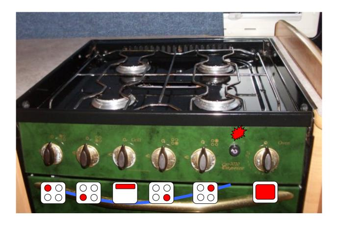
The knobs must be held in for a few seconds after lighting. This is a safety feature that turns off the gas if the flame blows out.
