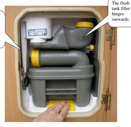
The flush water is replenished using the hosepipe, adding pink flushing additive at the rate of 30ml per 10 litres of water.
