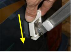
Then slide the latch down to lock the strut in place.
