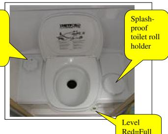
The outlet from the toilet bowl is normally closed with a black sealing "blade".
